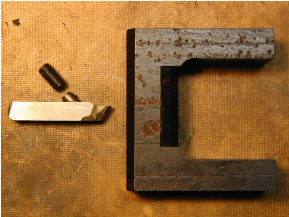
The clearance slot is located by inserting a new bit and scribing the top/bottom of the slot. Add an additional 50 thousandths for kicks and for any wear on the thrust bearing that will drop the cutting bit down.
