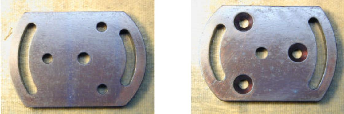
An adjustable stop plate was fabricated to mount on the top of the gearbox, as one can never have enough features. The following are pictures of the top and bottom views of the adjustable stop plate.
