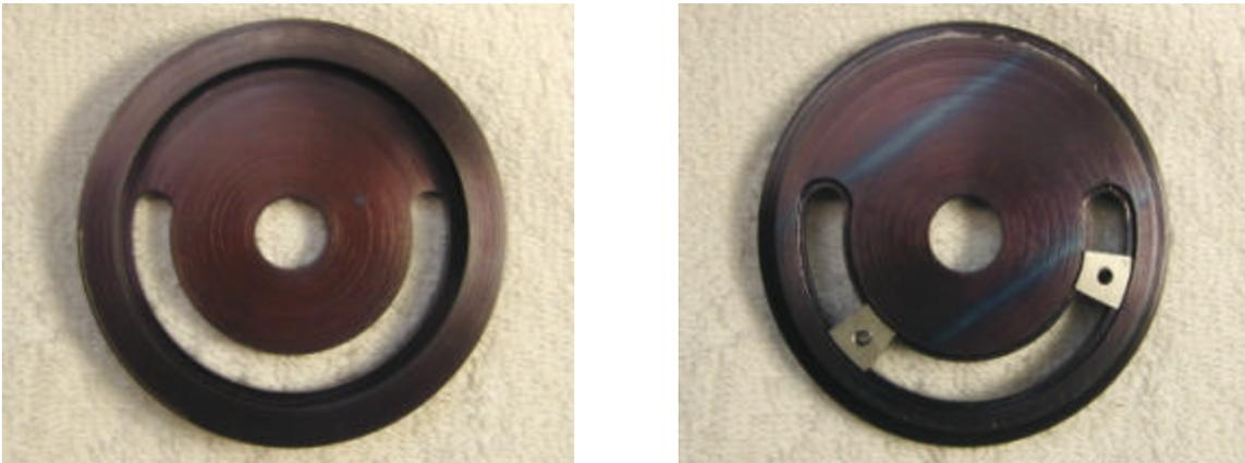
The T-nuts were milled out with the correct radius for the slot. They would probably be fine with parallel sides, but they fit and slide quite well with the mating curved sides.
